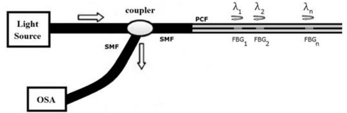
Fig. 4. Configuraiton of PCF-FBG acoustic sensor array for multipoint sensing.
