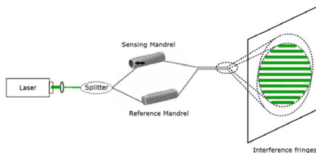
Fig. 1. Typical fibre optic interferometric setup to detect acoustic signal based on interference fringes.
