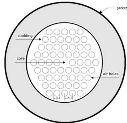
Fig. 2. Cross sectional view of a typical PCF fibre showing the characteristic structural features including air holes
