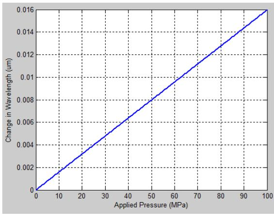
Fig. 6. Change in centre wavelength with applied pressure
