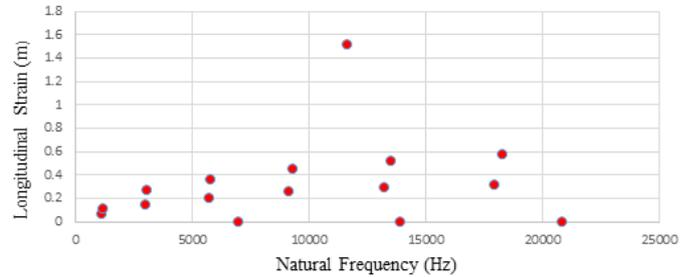
Fig. 8. Longitudinal strain for each natural frequency of solid cylinder.
