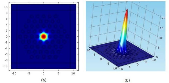
Fig. 5. (a) 2D and (b) 3D view of the electric field distribution profile of a 4-ring PCF.
