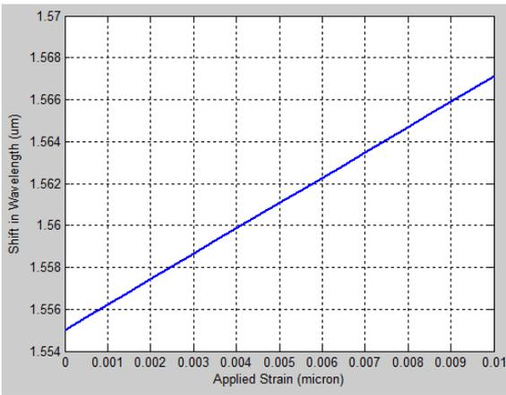
Fig. 7. Shift in Bragg wavelength for applied strain
