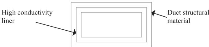
Fig. 10 A duct with a high conductivity liner.
