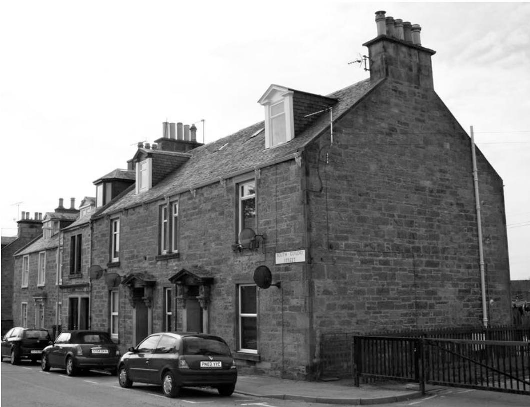
Figure 7. Comparable example from Elgin, Scotland. Image shows use of (originally) five sided dormer windows and gable chimneys. One should also note the use of chimney pots, similar to those in Lorrain's Tavern, Pictou.
